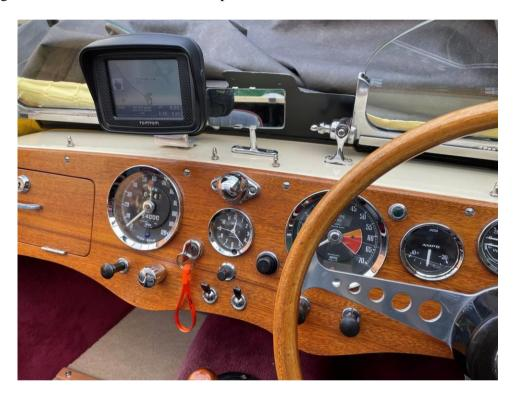
Originally Cracker must have had separate oil pressure and water temperature gauges as there is a newish combined oil/water gauge fitted, with an unserviceable oil pressure gauge filling the spare hole. A voltmeter gauge was purchased to replace the u/s gauge.
